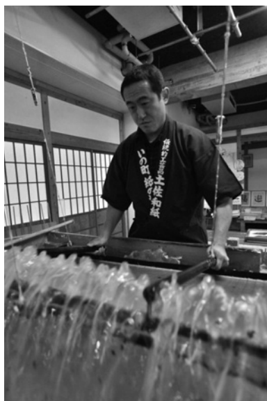
Nagashi-zuki (Scooping up the pulp stock) (Photo from Inomachi Paper Museum in Kōchi prefecture)
